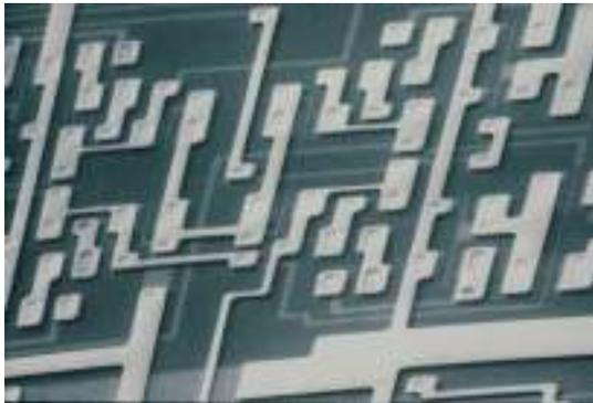
Fig. 8. The process featured passivated devices and fully-planar geometry made possible by proton isolation and polyimide intermetal dielectric.
