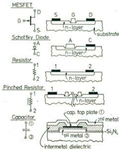
Fig. 7. The 1981 RFIC Process offered designers a complete set of components: MESFETs, Schottky Diodes, resistors and thin-film capacitors.
