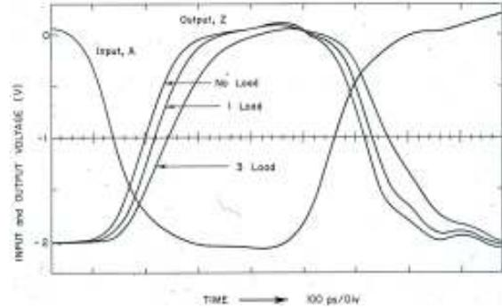
Fig. 3. The NAND/NOR logic gate showed 60ps delay with one output load, 75ps with two loads, 105ps with three loads.
