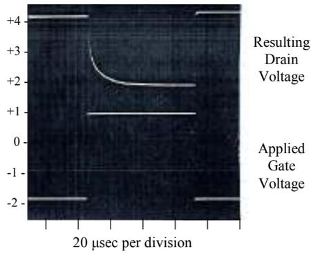
Fig. 1. On October 30, 1972, after joining HP Labs, I first discovered the *Lag Effect*. Since only 25% of the drain current responded immediately to a change in gate voltage, this rendered MESFETs useless as switches.
