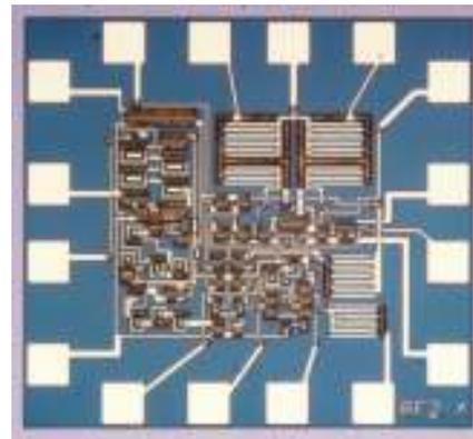
Fig. 6. The RF Signal Generation chip of 1978/79. The local oscillator tuned 2.1-2.5 GHz using on-chip tuning diodes and an off-chip inductor. The downconverted I.F. was dc - 1.4 GHz.
