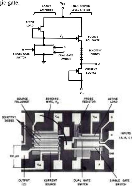
Fig. 2. The world's first GaAs MESFET logic gate, 1973.
