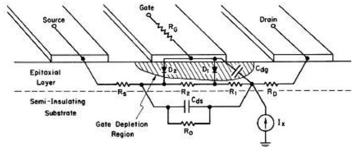
Fig. 4. The 1974 non-linear MESFET device model was based on a 2-lump approximation of the FET channel. Pinchoff was proportional to square root of gate voltage, but velocity saturation - approximated by the hyperbolic tangent function - mimicked the short-channel properties of the MESFET. This model became a key tool for subsequent IC design [21].
