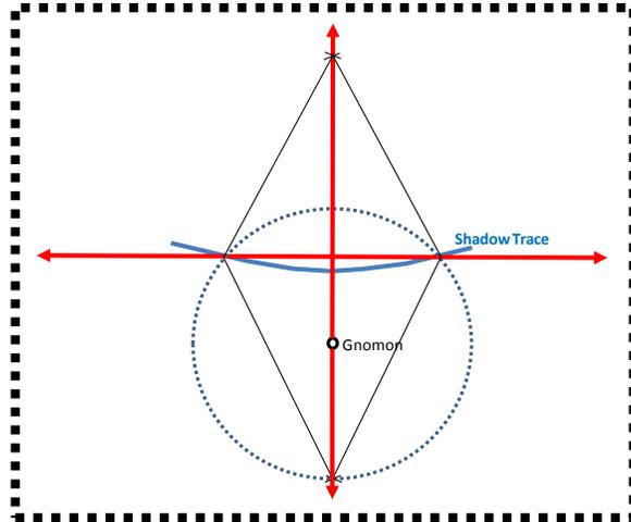
Fig. 5. The East-West and North-South baselines are determined as shown, using the solar method
