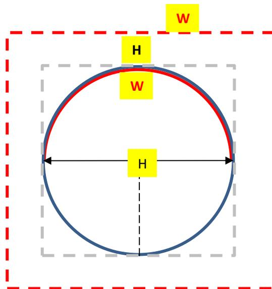
Fig. 4. The rope of length  $W$  defined the base dimension of the Great Pyramid.  $H$  was the desired height. This method was possibly chosen for reasons of mystical significance. But the height to base ratio was greater than that of the somewhat squat Red Pyramid, and by coincidence was close to the so-called “Golden Ratio” used in later Greek architecture.
