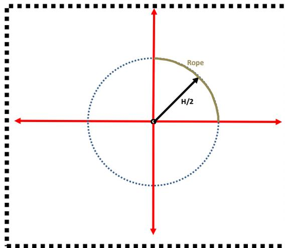
Fig. 6. A circle of diameter equal to the design height of the pyramid is inscribed with center at the intersection of the baselines. A rope is laid along one quarter of this circle to create a tool for the following steps.
