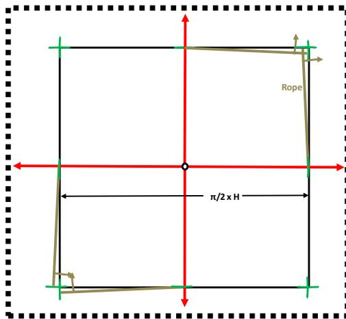
Fig. 8. The rope is used to mark the corners of the square pyramid base. The square is inscribed. They then had a north-south oriented square of side equal to  $\pi/2$  times the design height, and the center of this square was marked for reference.
